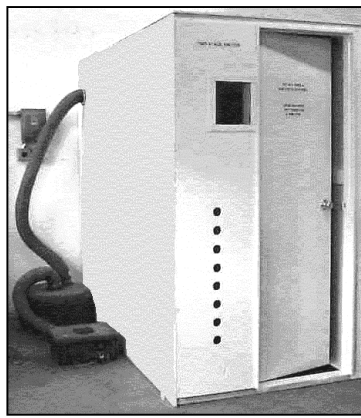
Figure J-5. Fabricated Airlock with Filter-Blower Unit
